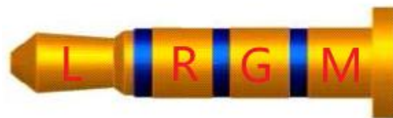
Figure 15 Definition of four-segment headphones
