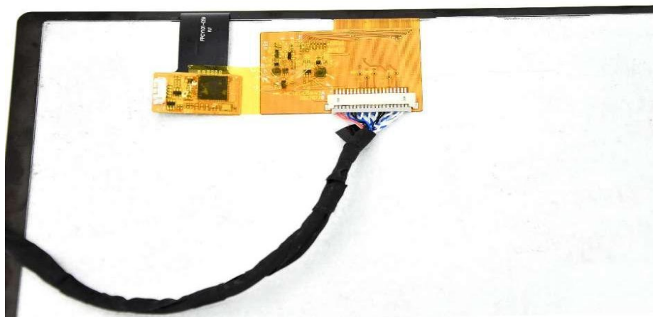
Figure 31 Connect LVDS screen cable to LVDS screen
